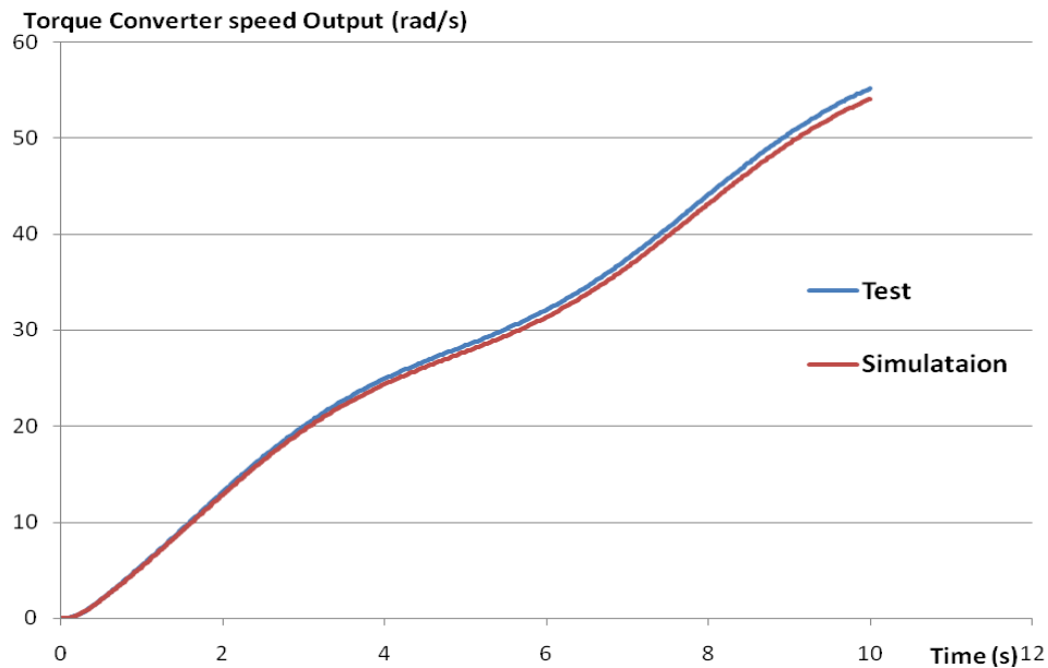
Figure 6-12 Torque Converter Validation - Output Speed
