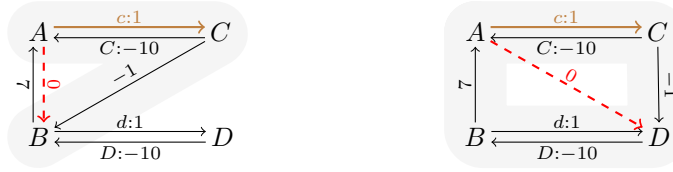
■ Figure 1 A semi-reducible path (shaded gray on the left) and a Semi-Reducible Negative (SRN) cycle (shaded gray on the right).
