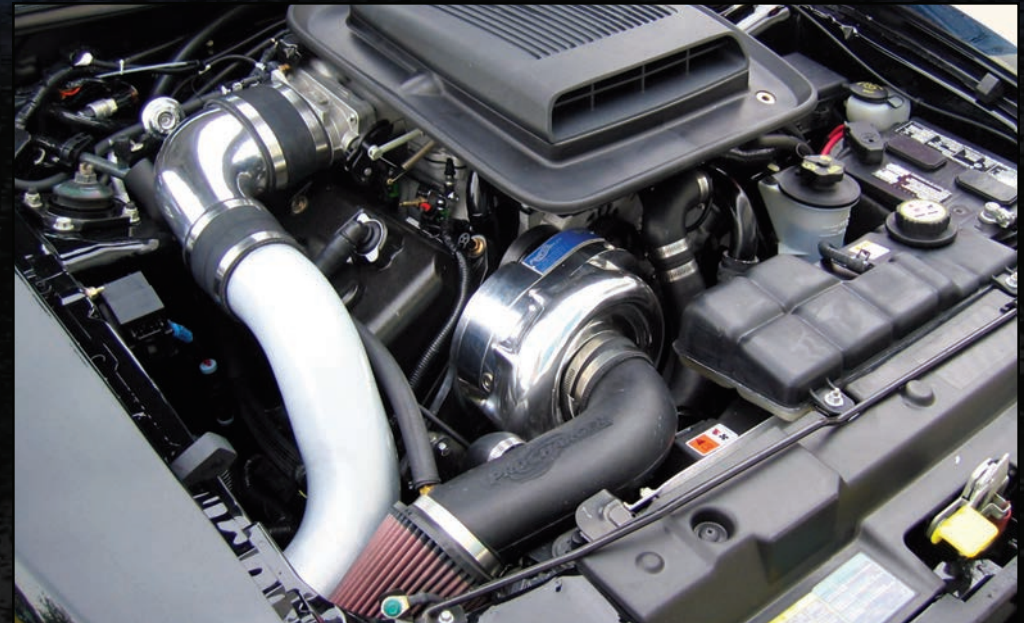
The ProCharger Mach 1 Stage II Intercooled System retains functional air scoop
