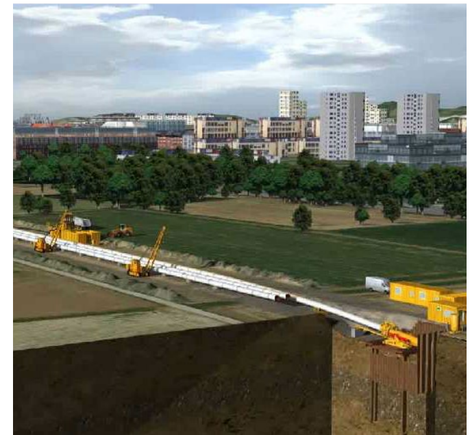
ABOVE: We have approximately 40 major trenchless crossings planned for the Expansion Project. They greatly mitigate impact to normal daily activities and traffic circulation patterns, and minimize or eliminate ground disturbance.
