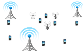
Fig. 1. HetNet is comprised of macro nodes and small nodes. Data traffic on the edge of macro cells are offloaded to the small cells, so that the performance on the macro-cell boundary area is improved and traffic load for the macro cell is alleviated.
