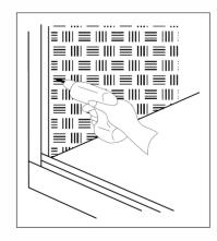
the framing timber. Use the 4mm drill bit to drill holes through the glass receiver channel. Fix four screws through the channel in the wall framing (use wall plugs if required).
