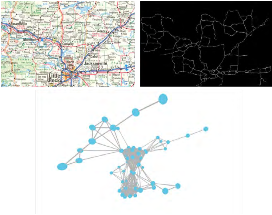
Figure 1. Sample of image input (upper left), internal output (upper right), and final graph as produced by Histonets (lower)
