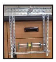
The class will also develop different truss designs and use a tensile tester (pictured) to test the strength and develop an understanding of all the stress and strain points within a truss.
