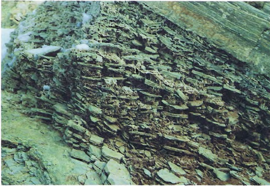
32. Example of expanded bedding planes with gypsum filaments in unit 4 located approximately 800 feet downstream of dike.
