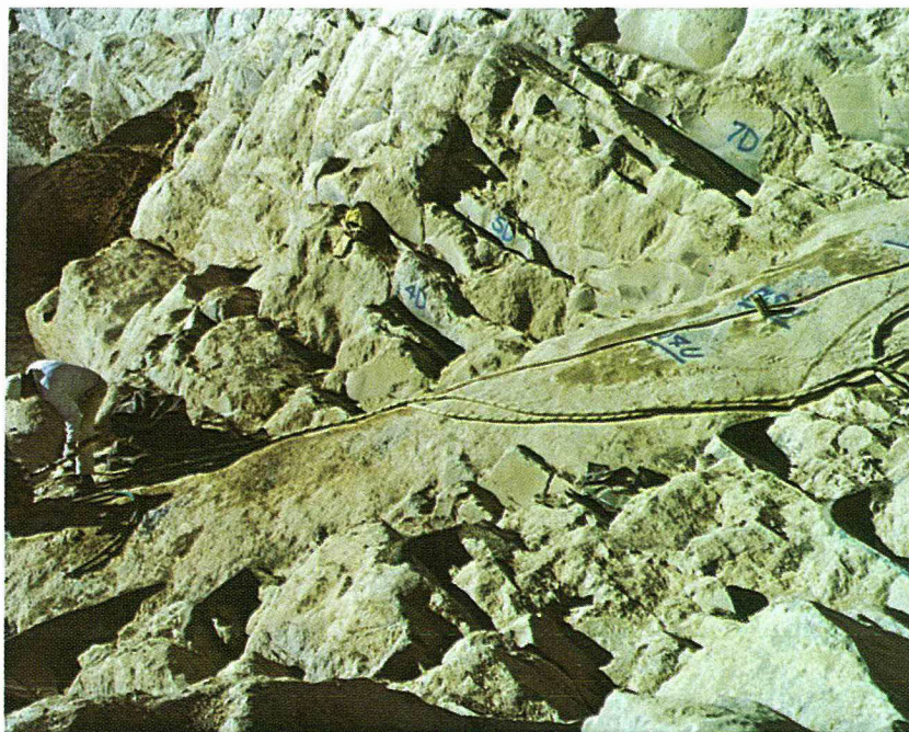
Fig. 3-16 Test ponds for joint transmissibility tests, looking downstream
