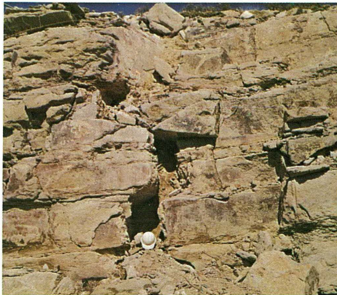
Fig. 5-20 Joint in right wall of Teton Canyon 1/8 to 1/4 mile upstream from dam. (post-failure photo)
