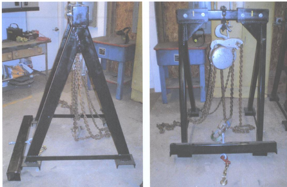
Figure 2-6: Spillway Gate A-Frame Hoisting System (Boyce Hydro 2012b)
