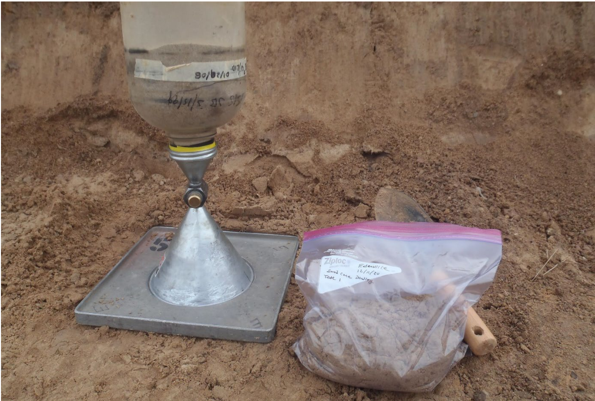
Figure E-6: Sand Cone Density Test Performed at the Left Embankment Remnant
