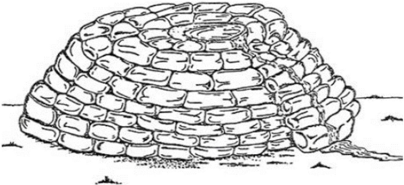
Figure 21: Sketch of a Typical Sandbag Ring Levee with Spillway
