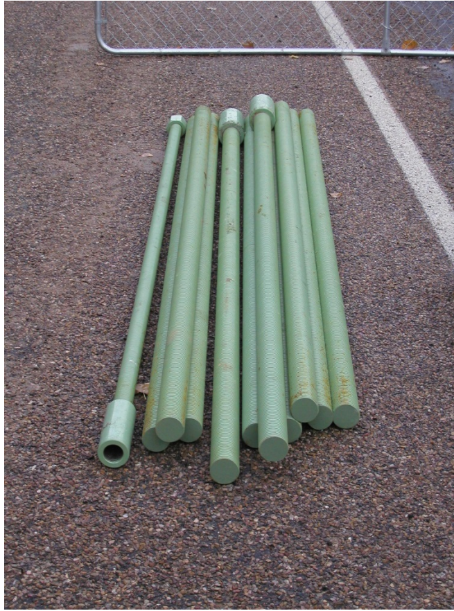
Figure 14-5.—Epoxy coated rock bolts (Reclamation).
