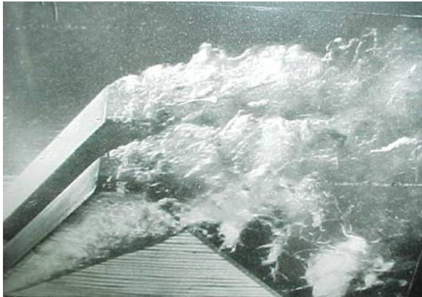
Figure 3-9.—Cavitation created in low ambient pressure chamber (Reclamation, 1990a).
