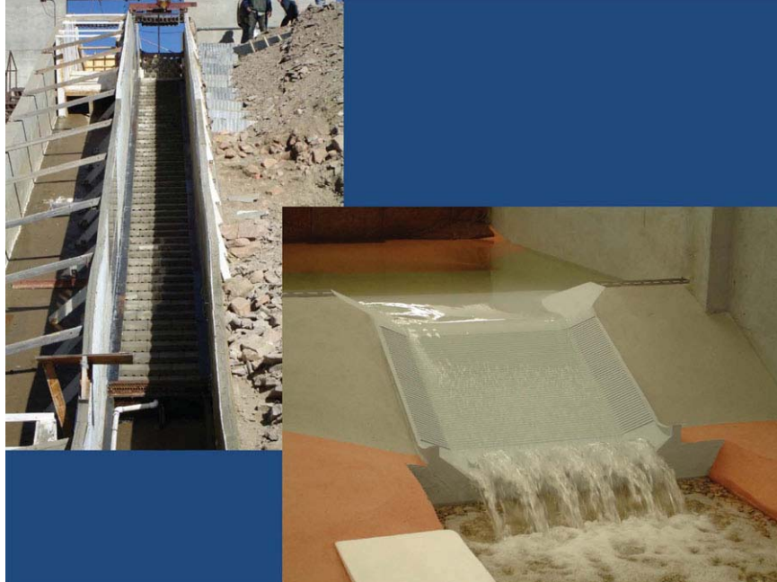
Figure Barriga-2.—(a) Prototype two-dimensional flume testing of the standard ArmorWedge block performance at CSU (upper left) (courtesy of CSU).
