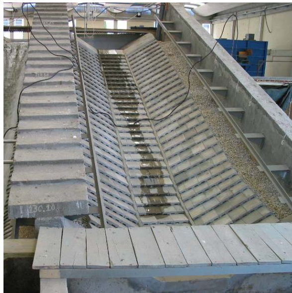
Figure Barriga-3.—Laboratory testing of smaller scale wedge-shaped blocks in a trapezoidal channel over a compacted embankment in Portugal. General testing of velocities, air concentration, depths, pressures on the surface and in the drainage layer, and drainage flows have been accomplished with the data used for the Barriga project (courtesy of LNEC, Portugal, all rights reserved).
