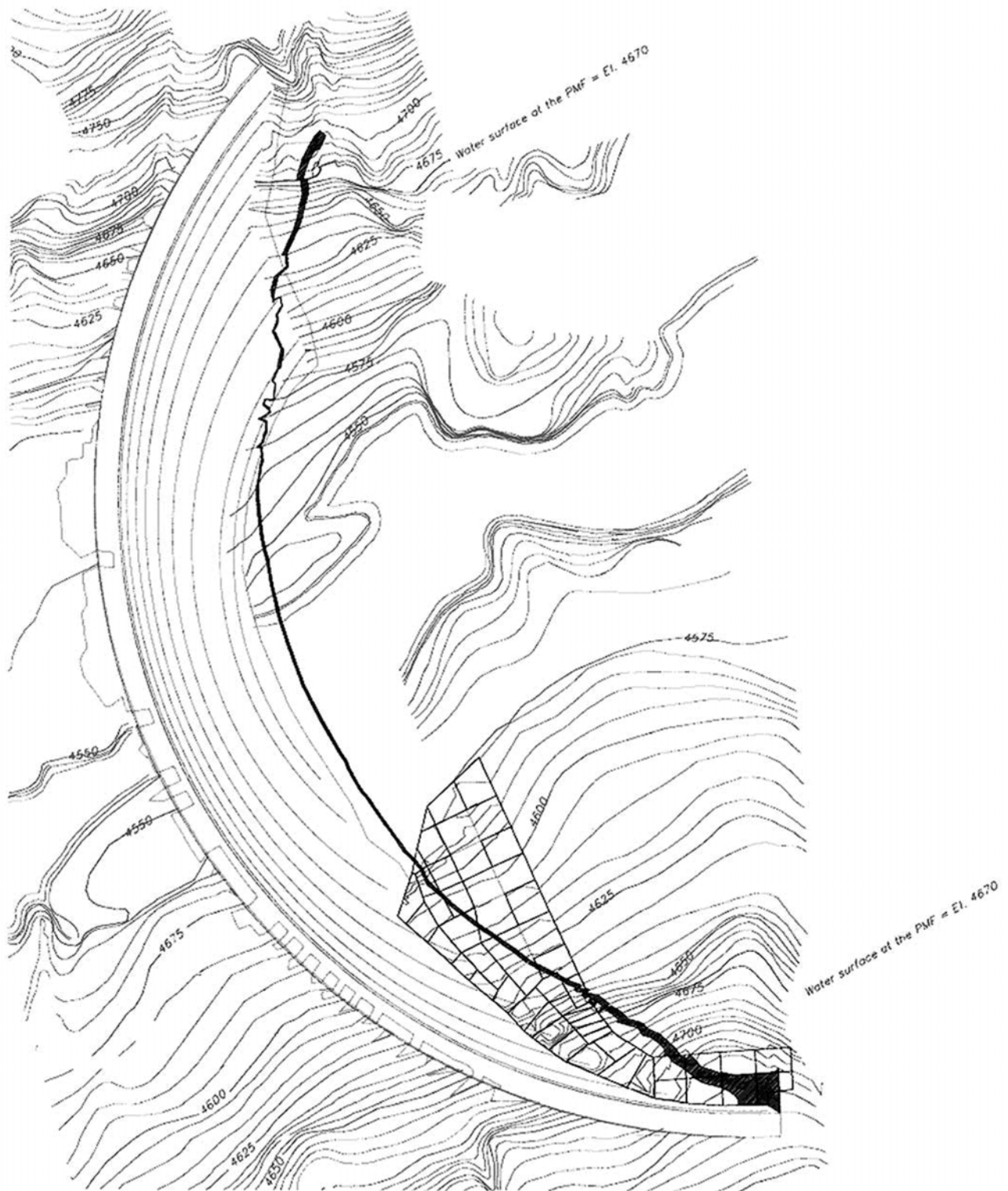
Figure 11-4.—Footprint of the trajectory with no spread of the jet for the PMF overtopping. Note the location of the footprint extends beyond the right abutment protection between contour elevations 4660 and 4710. The tailwater for the PMF is shown on the plan view in blue at Elevation 4670 (Reclamation 2006).
