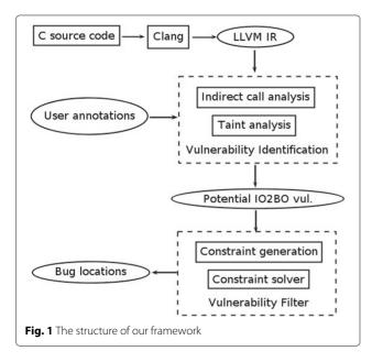
taint sources and sinks are given by our built-in annotations as well as user annotations. Potentially vulnerable integer operations are identified by the comparison with the pattern of IO2BO vulnerabilities; the second stage performs constraint generation and solving for each potential IO2BO vulnerability, if the constraint of a potential IO2BO vulnerability cannot be satisfied, the vulnerability will be filtered out, which helps reduce false positives.
