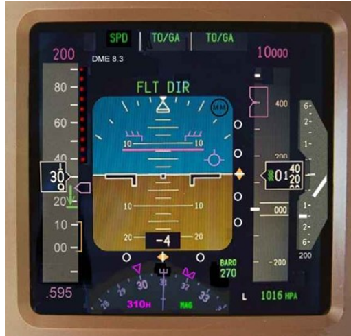
Figure 1: Primary Flight Display of a Boeing 777
