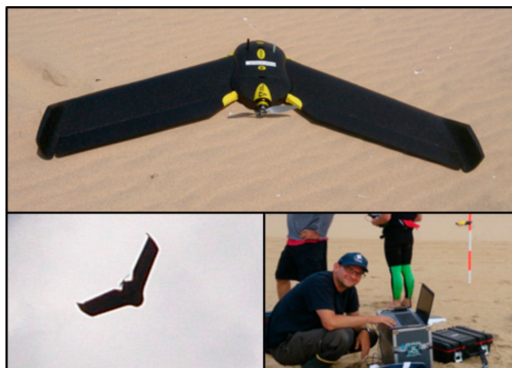
Figure 2. eBee UAV during a field campaign, in flight and the hardware.
