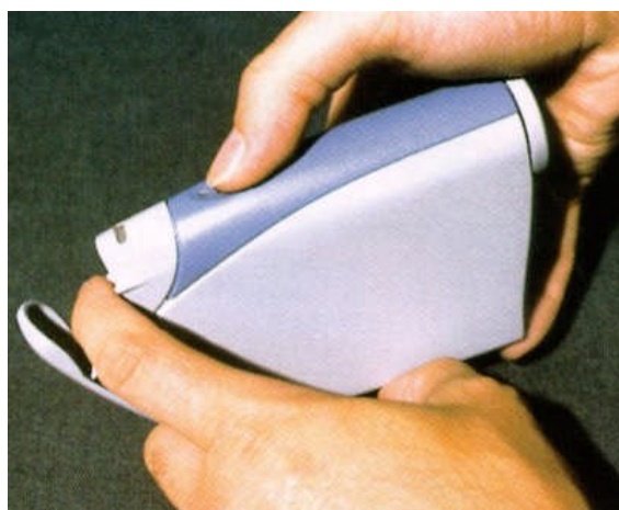
Figure 25: Cell Robotics Lasette® Laser Ablation Blood Sampling Device
