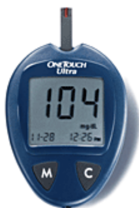
Figure 13: OneTouch Ultra Blood Glucose Biosensor
