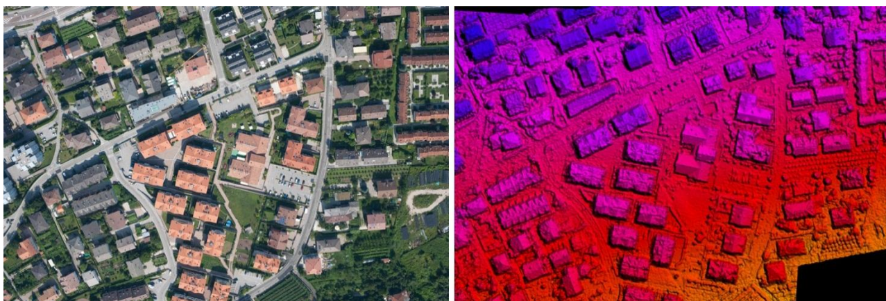
Figure 3. Automated DSM generation (25 cm geometric resolution) from aerial images acquired with a SLR camera from a helicopter (10 cm GSC).
