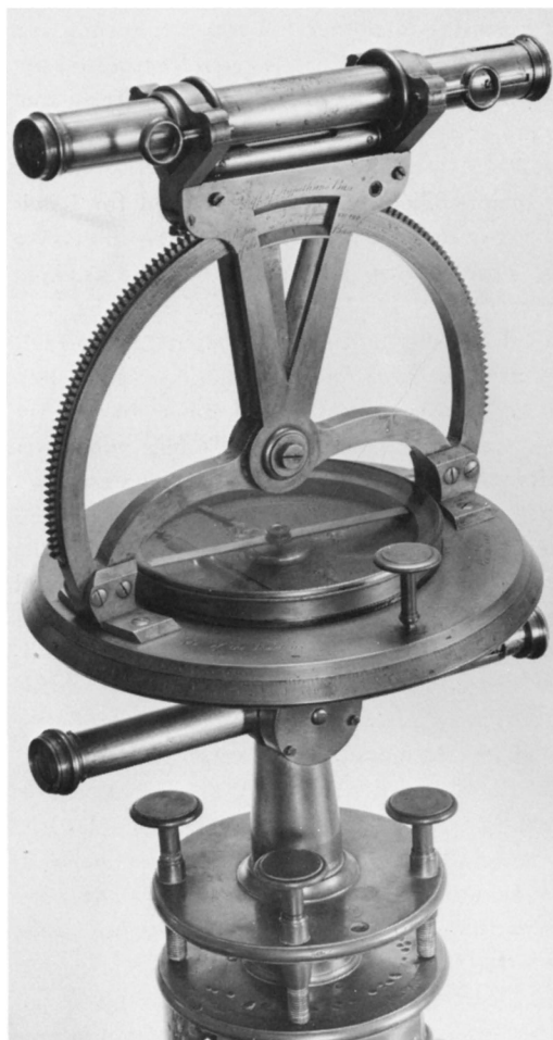
FIG. 2. Equatorial theodolite made by Jesse Ramsden, London, owned by Thomas Jefferson. (Thomas Jefferson Memorial Foundation)
