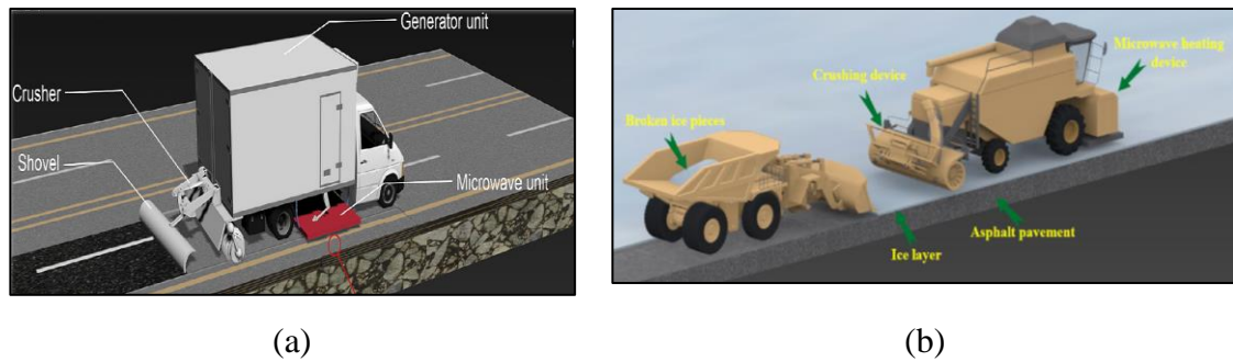
Figure 3.10 Schematic diagram of (a) an all-in-one mobile microwave deicing unit 1 and (b) a mobile microwave deicing unit that uses two vehicles 85 .
