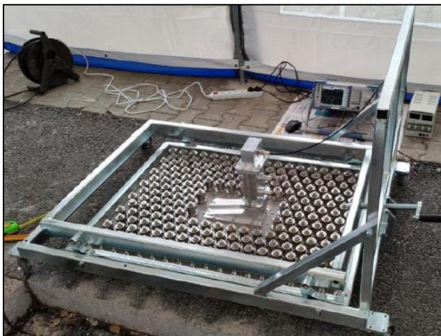
Figure 2.7 Microwave applicator with leakage suppressing choke. 56
