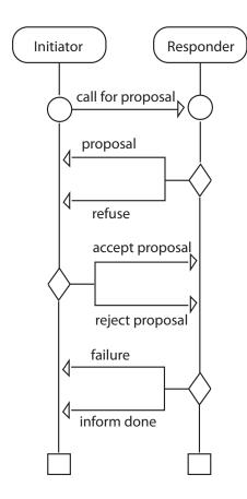
Figure 3: One of the agent interaction protocols that we implemented to support communication in our agent architecture (the FIPA Contract Net Interaction Protocol).
