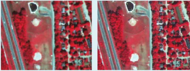
Panchromatic merge using Quickbird imagery—multispectral at 2.4 meters, panchromatic at 0.6 meters. Raw image is on left. Image on right is after the merge. Note the increased spatial resolution and heightened texture.
