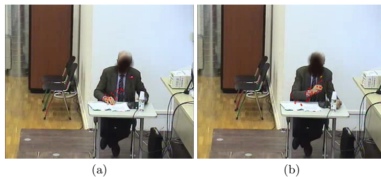
Fig. 7. SURF feature points found in the video after it is masked by the Activity Area.
