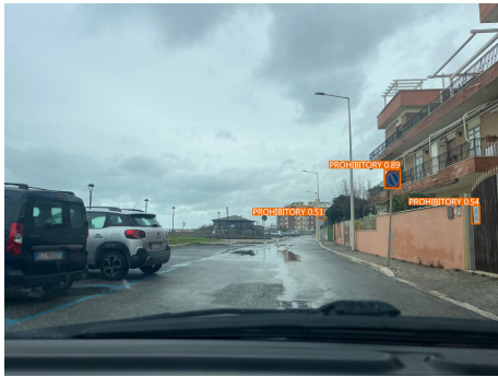
Figure 6: Frame extracted from the PDD dataset predicted by the fine-tuned model YOLOv8. The predicted traffic signs and the correlated label and accuracy are highlighted in orange.
