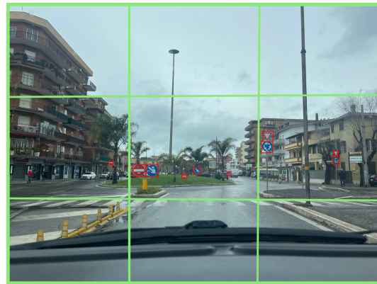
Figure 1: Example of an external image after road signs detection, with the ROI grid in green. Several regions of interest which contain one or more road signs have been identified in the image (specifically, cells 4, 5 and 6). The red rectangles represent the traffic signs bounding boxes.
