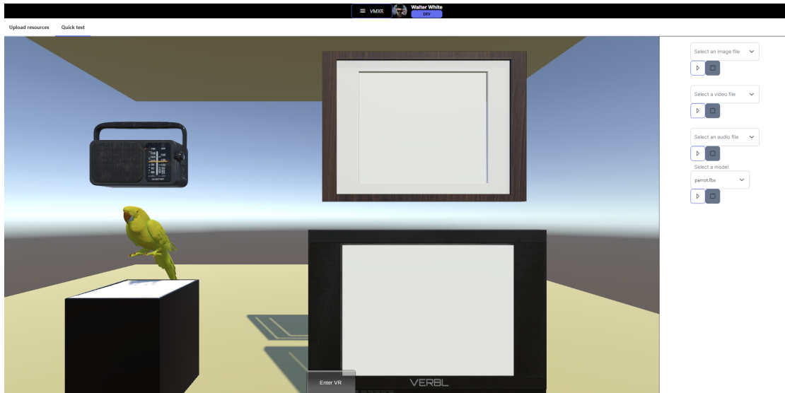
Figure 1: Four sample objects uploaded by a Dev for supporting EC and XC in creating the XR environment. Each one is associated to one or more Unity components providing high-level actions (e.g., play sound for the radio, play video for the screen etc.)
