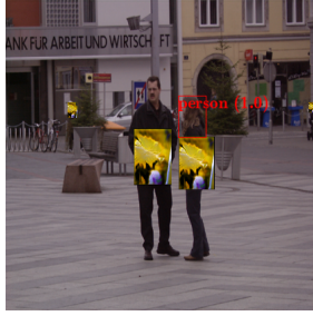
Figure 13: A naturalistic patch, created using the framework by Hu et al. [5], attacks objects of the class person via overlapping with the clothing area
