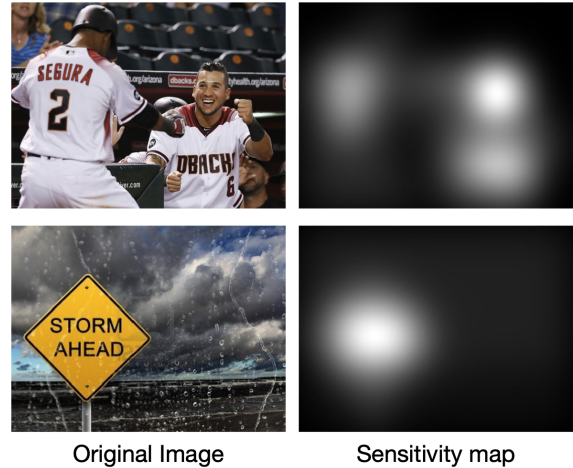
Figure 1: The figure shows sensitivity map examples. The left column has the original images and the right column are the corresponding sensitivity maps. For example, in the first image, its sensitivity map highlights the humans, indicating that noise added to the human region will be perceived more easily than when the noise is added to the background.
