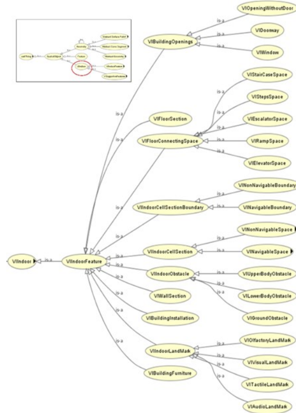
Fig. 1. Top Level Ontology for VI building features (inset shows the link with geometry class)
