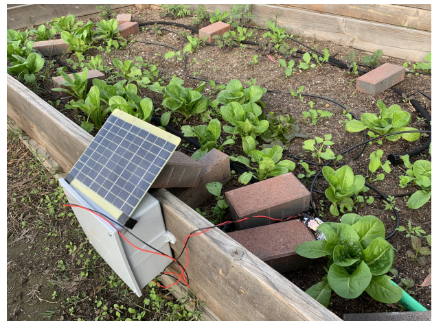
Fig. 4. Set-up of the garden experiment with sensors and automated watering
