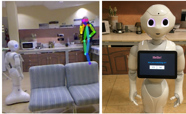
Fig. 3. Monitoring the user activity by indirect observation (left), or by making a request (right)
