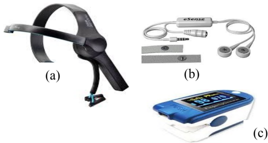
Figure 3: Data collection devices: (a) Neurosky EEG device (b) GSR device from eSense (c) Pulse oxymeter from Contec
