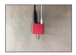
**2.** Connect any pair of headphones. The mic channel is not available on the second connector.
