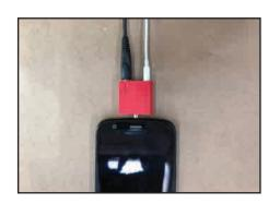
**3.** Plug Rockit into your phone's combo jack. Audio goes out through the second connector, and mic or other input comes in through the first connector. **Note:** for best results, always plug accessories into Rockit before connecting to your phone.
