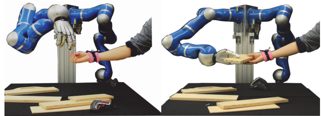
Figure 1: In this paper a robot collaborator must decide which action it should take in a proactive manner, before the human requests such action. We motivate the method with an experiment of a collaborative toolbox assembly where the robot must anticipate if the human will ask for a plate or for a screw.
