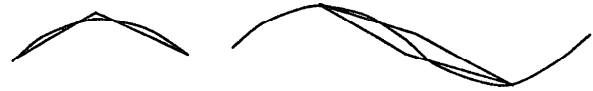
Figure 13: (Left) Single arc case: both ends of the link pair are on the same cubic spiral. (Right) Tangent arcs case: both ends are on consecutive cubic spirals with opposite sign of curvature. Tangent arcs with the same curvature sign is similar to the single arc case and is less critical.
