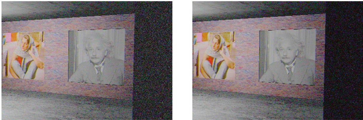
(a) Weighting function of Debevec et al.: PSNR = 25.70dB. (b) Prob. weighting function PSNR = 28.59dB.
