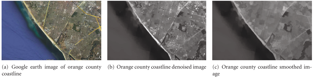
FIGURE 4: This shows how we obtained our valid region for the Orange County Coastline example. Figure (a) is the initial aerial image of the region to be considered. The region of interest is about 15.2 km by 10 km. Figure (b) is the denoised version of the initial image. We took this denoised image and smoothed away from regions of large discontinuities to obtain figure (c).
