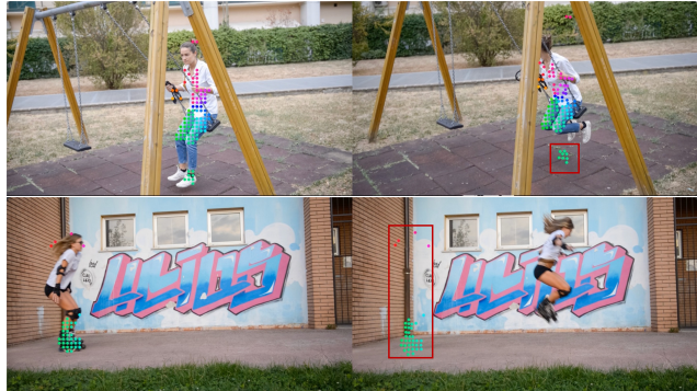
Figure 5: Erroneous correspondences after cycle consistency check. The red bounding box highlights a common type of incorrect correspondences from flow networks like RAFT [66] that remains undetected by cycle consistency check. The left images are query frames with query points and the right images are target frames with the corresponding predictions. Only correspondences on the foreground object are shown for better clarity.
