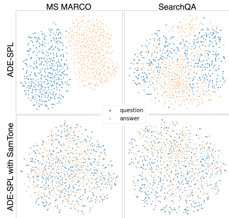
Figure 1: Embedding space analyses on MS MARCO and SearchQA show that sharing a projection layer in Asymmetric Dual Encoders (ADE-SPL) (Dong et al., 2022) may not guarantee that the embeddings from the two encoder towers are in a coinciding parameter space. However SamToNe can effectively achieve that.
