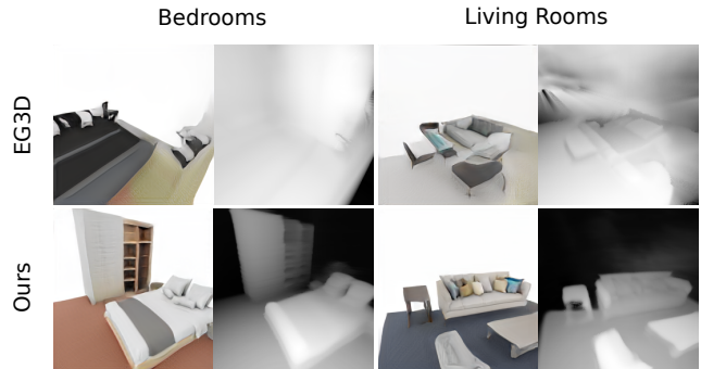
Figure 7. Visualization of depth maps – extracted from the density fields. Our method is able to generate sharp depth maps in comparison to EG3D, which produces unrecognizable results.
