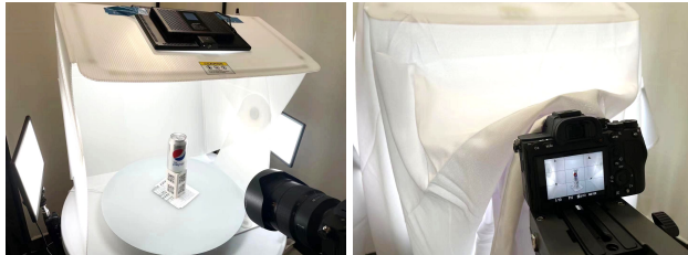
Figure 3. (Left) We use a light box with controllable lighting for our capture. To mitigate near-field reflections, we leverage a thin stand to support the object. (Right) To minimize environmental changes due to camera and photographer movement, we cover the lightbox with a cloth and use a turntable for multi-view capture.
