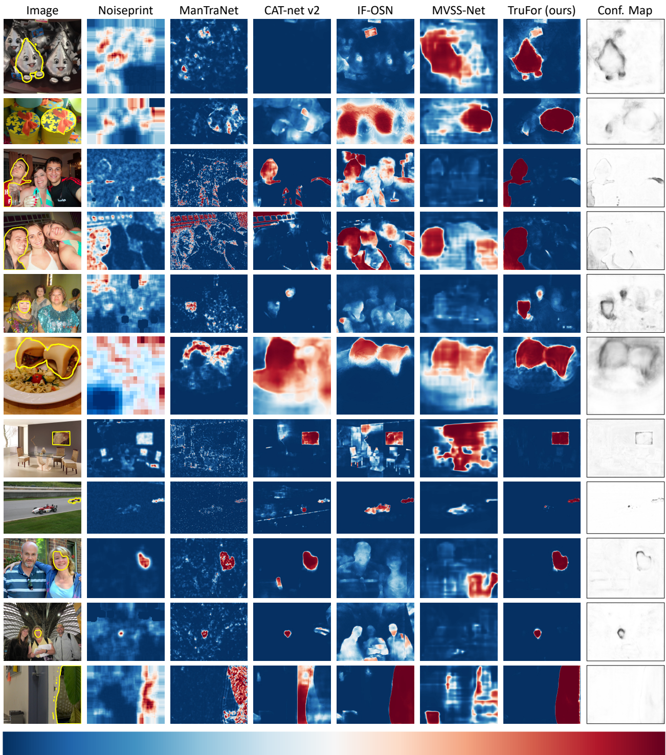
Figure 13. Some qualitative results, compared with the state-of-the-art, on manipulated images (the forged area is outlined in yellow). Dark regions in the confidence map indicate regions of low confidence in the TruFor localization map.
