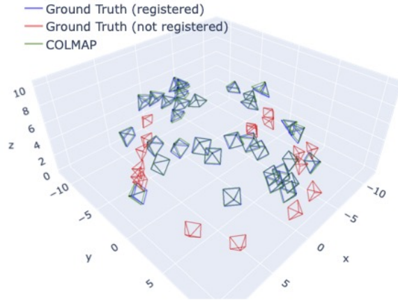
Figure 16. COLMAP – Camera positions recovered by COLMAP (oriented towards zero-center solely for visualization). For images with estimated camera pose, COLMAP’s estimates (green) are extremely close to the ground truth (blue). COLMAP failed to pose ground truth cameras in red.
