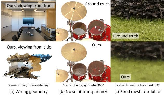
Figure 8. Limitations – (a) the monitor/table are hollow, because the reflections are modelled as real objects behind the monitor and below the table. (b) our method generates scattered small fragments in the semi-transparent parts. (c) the camera is too close to the scene and details in the grass cannot be represented at the chosen texture resolution.
