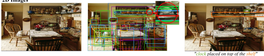
Fig. 1: Language-modulated 3D (top) and 2D (bottom) detection with BUTD-DETR. Middle: State-of-the-art object detectors often fail to localize small, occluded or rare objects (here they miss the clock on the shelf and the bottle on the cabinet). Right: Language-driven and objectness-driven attention in BUTD-DETR modulates the visual processing depending on the referential expression while taking into account salient, bottom-up detected objects, and correctly localizes all referenced objects.
