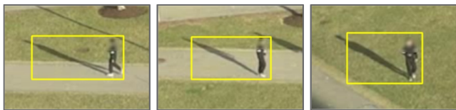
Figure 19: The shadow of the target object could be considered as a part of the target object because they have the same motion.
