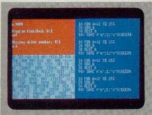
The screen format for the input/output of YS MegaBasic . Three windows are provided for input, LISTing and RUNNING programs; under software control, each window's size and purpose can be changed to suit individual requirements.
