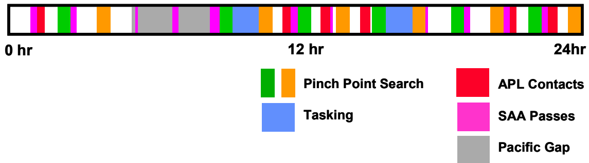
Figure 9. Schedule of twelve pinch point data collection periods subject to operational constraints. It is possible to schedule the data collection to avoid APL contacts and minimize data collection in the SAA and of the Pacific gap.
