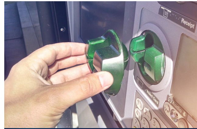
A skimmer being installed on an ATM Source: Washington State Department of Financial Institutions
