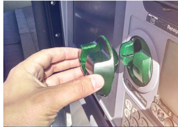
A skimmer being installed on an ATM. Source: Washington State Department of Financial Institutions
