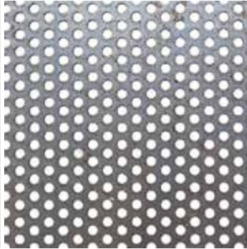
A606-4 (aka Corten®)* 22 GA / 20 GA PERFORATED PATTERN - .127 Round & 7/32" Stagger - 30.58% Open Area
