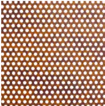
Corten AZP Raw® 24 GA PERFORATED PATTERN - .127 Round & 7/32" Stagger - 30.58% Open Area
